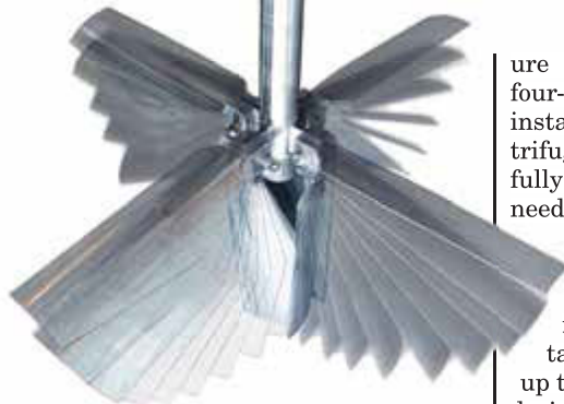
FIGURE 6. Sharpe Mixers offers a folding blade impeller, which features a hydrofoil-style, four-blade design that folds for easy installation and opens with centrifugal force, locking in place when fully opened
