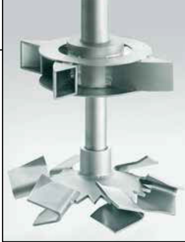
FIGURE 4. Because hydrogenation processes were traditionally limited by mass and heat transfer, and because the hydrogen is difficult to handle and such reactors must be operated absolutely gas-tight at high pressures, Ekato developed a self-aspirating gassing turbine, which is specifically applied in such reactions to overcome the mass-transfer limitation
