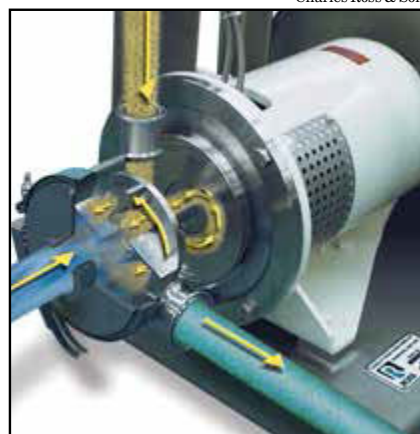
FIGURE 5. Charles Ross & Son’s SLIM Solids Injection Technology consists of a rotor and stator mixing arrangement, specially designed to create negative pressure (vacuum) behind the rotor
